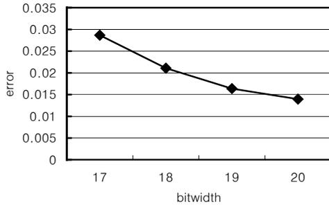
**Fig. 2 The RMS error for varying bitwidths**
