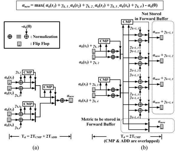
Fig. 3. (a) Conventional and (b) retimed ACS block with four operands.
