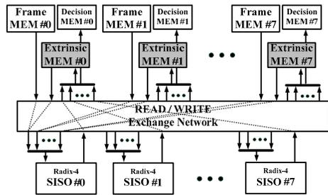
Fig. 2. The proposed chip architecture with eight SISO decoders
