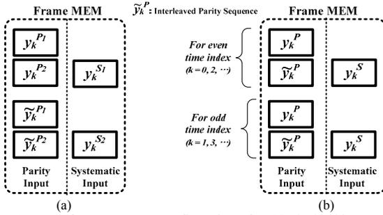
Fig. 4. Input frame memory configurations for (a) double-binary turbo decoding mode and (b) radix-4 single-binary turbo decoding mode.
