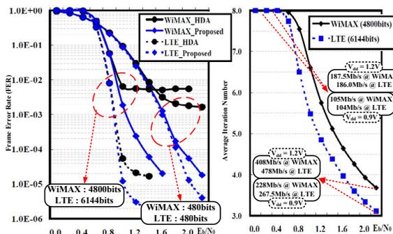
Fig. 6. FER performance and average iteration number with early termination in an AWGN channel.
