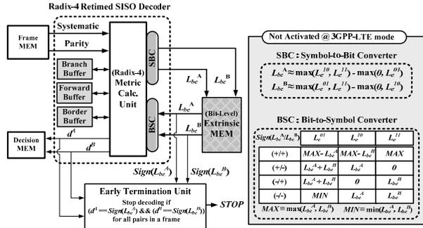
Fig. 1. Overall unified turbo decoder architecture with time-multiplexing
