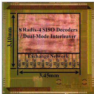
Fig. 7. Micrograph of the chip.
