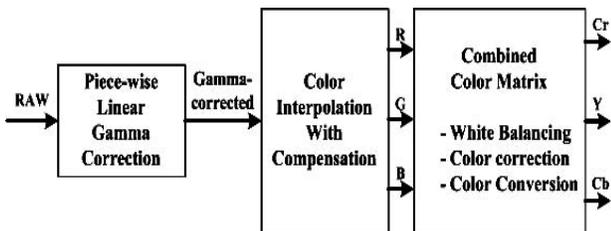
Figure 2. Proposed Image Signal Processing Structure
