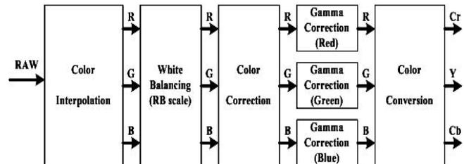
Figure 1. Conventional Image Signal Processing Structure
