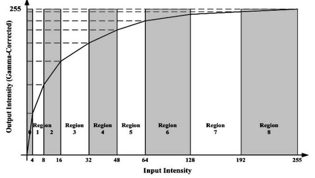
Figure 3. Piece-wise Linear Gamma Correction
