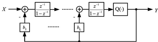
Fig. 1.  $L^{\text{th}}$ -order  $\Sigma\Delta$  modulator.
