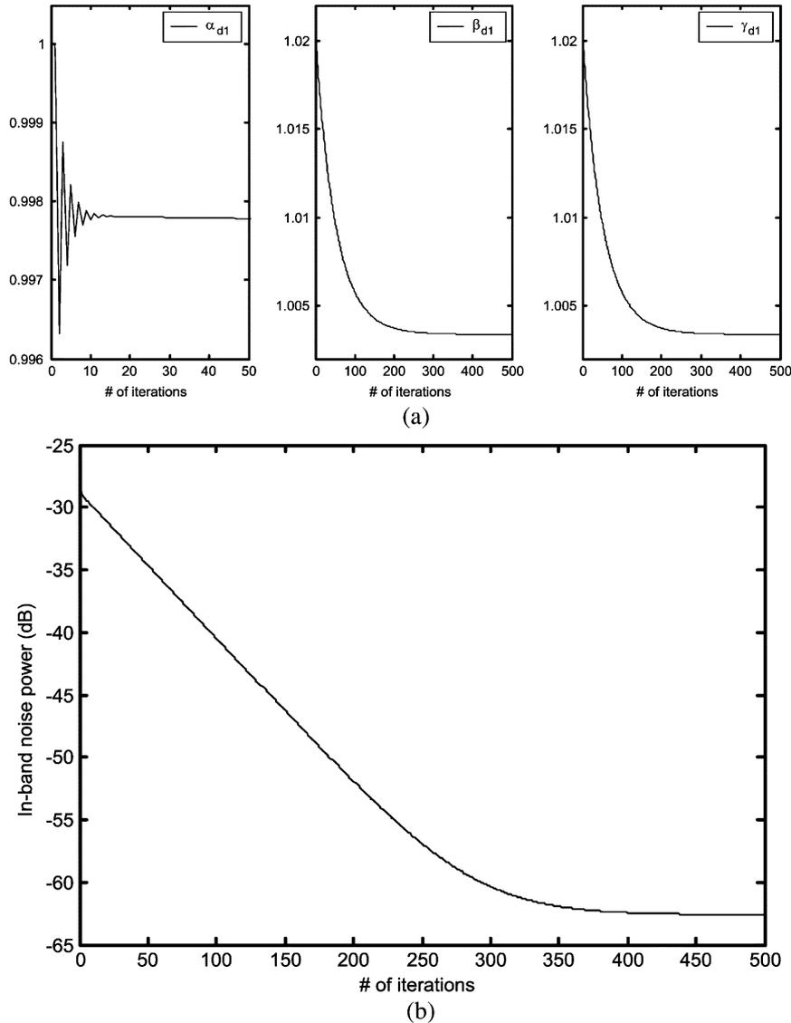
Fig. 10. Learning curve example for (a) digital gain coefficients and (b) the in-band quantization noise.
