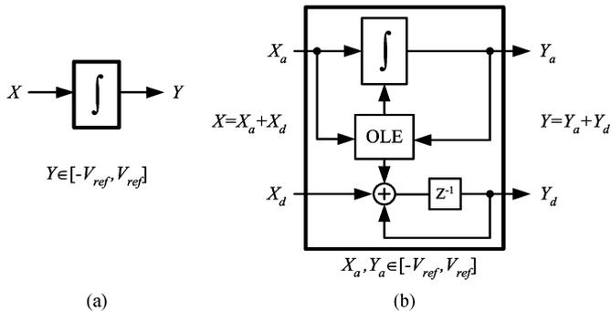
Fig. 2. Block diagrams of (a) analog integrator and (b) hybrid integrator.
