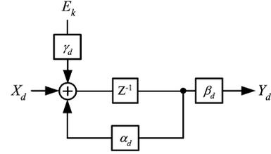
Fig. 8. Digital integrator with gain coefficients.
