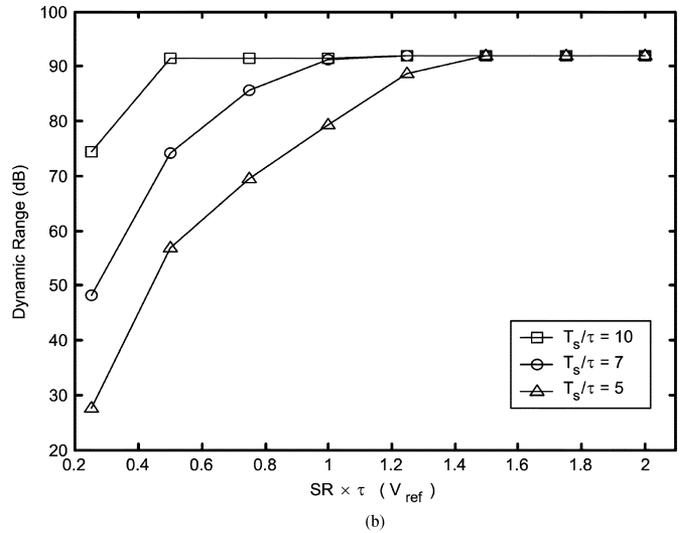
Fig. 13. Influence of integrator nonlinearity on the fourth-order hybrid  $\Sigma\Delta$  modulator with a 1-b quantizer: (a) input-dependent gain and (b) slew-rate limited settling.
