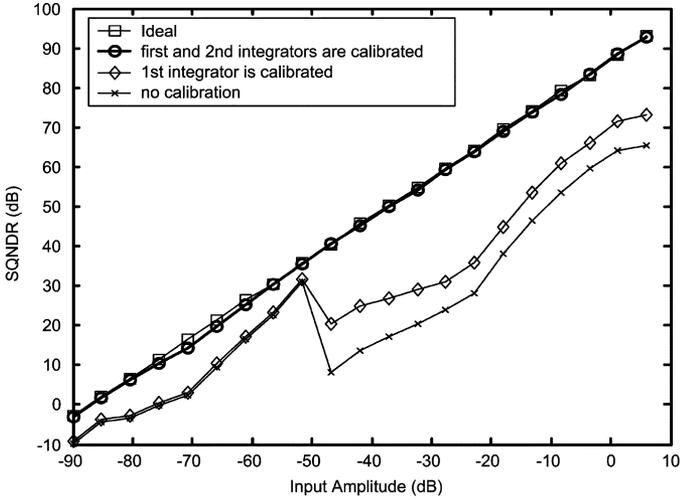
Fig. 11. SQNRs for different input levels of fourth-order hybrid  $\Sigma\Delta$  modulators with a 1-b quantizer.
