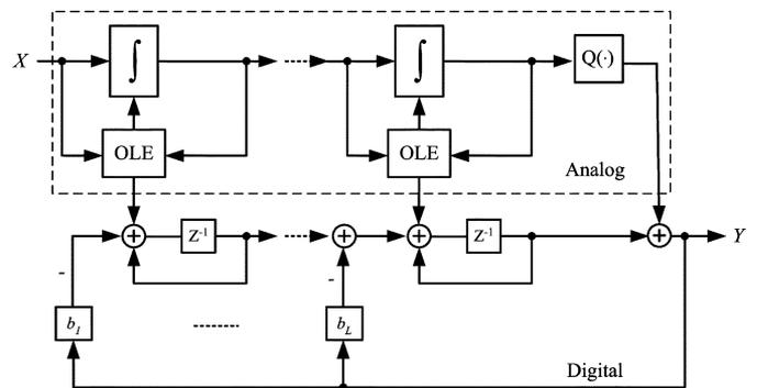
Fig. 3. Hybrid  $\Sigma\Delta$  modulator.
