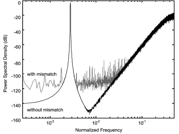
Fig. 7. Output spectra of a fourth-order hybrid  $\Sigma\Delta$  modulator with and without mismatch.
