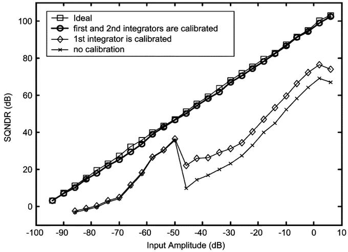
Fig. 12. SQNRs for different input levels of fourth-order hybrid  $\Sigma\Delta$  modulators with a 3-b quantizer.
