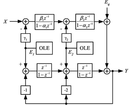
Fig. 6. Second-order hybrid  $\Sigma\Delta$  modulator with analog circuit imperfections.
