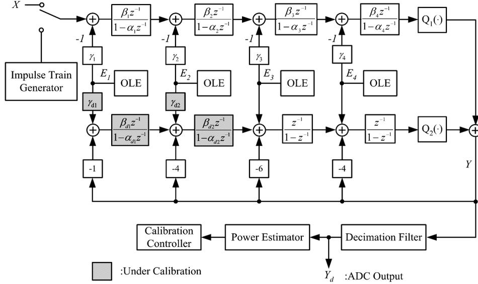
Fig. 9. Fourth-order  $\Sigma\Delta$  ADC with the proposed calibration technique.
