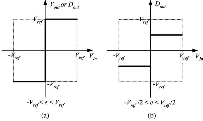
Fig. 5. 1-b quantizers of (a) conventional modulators and (b) hybrid modulators.
