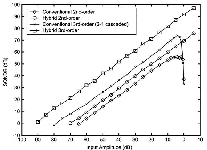
Fig. 4. SQNRs versus input amplitudes of  $\Sigma\Delta$  modulators (OSR = 32).
